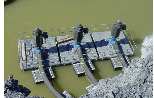
Large vertical pump with walkway.
